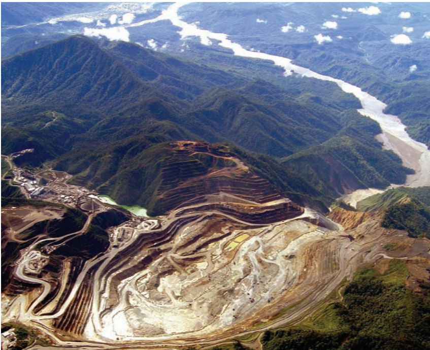
Figure 10 A view to the SE across the Ok Tedi mine open pit. Waste rock from the pit is discharged into the Ok Mani River which joins the Ok Tedi River at top left. The mine mill is in the small valley at left centre. Photograph: Ok Tedi Mining Limited.
